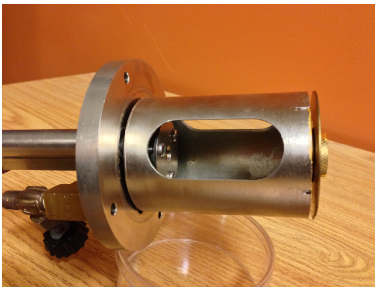
Figure 3: This image shows the cage with alpha source and gold scattering foil. Here the brass shield and plug assembly (including washer for spacing away from the gold foil) has been inserted in front of the scattering foil for calibration. The plug has a hole in the middle to form a direct alpha beam, and this can be covered with gold foil to fully simulate the energy loss in the gold foil scattering experiment.
