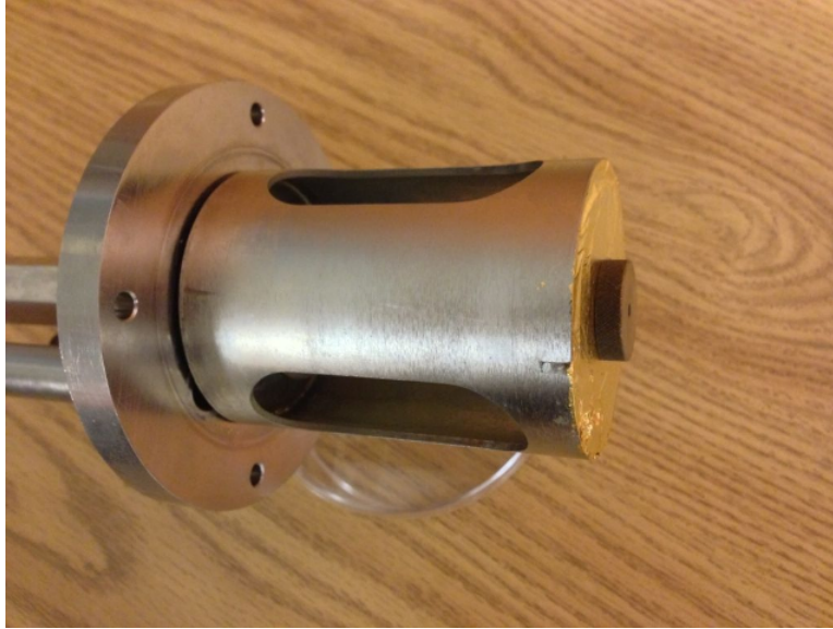
Figure 4: This image shows the cage with alpha source and gold scattering foil prepared for a scattering run. Here only a central plug (without hole) has been inserted.
