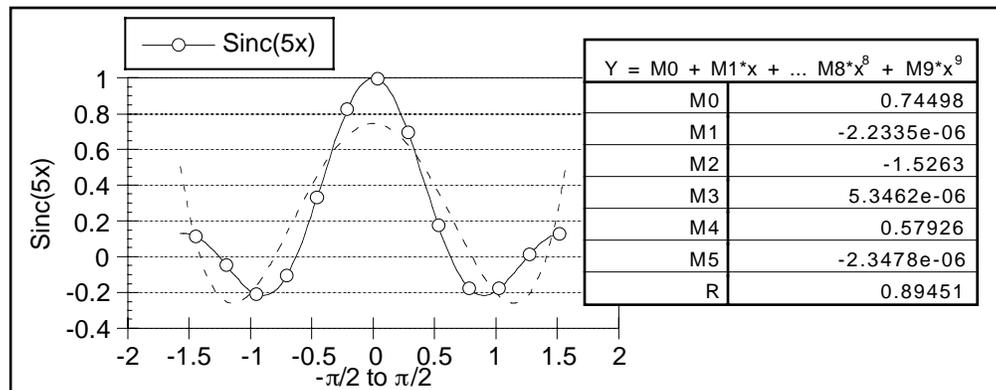
Figure 9-4 Sample plot with Polynomial curve fit applied
