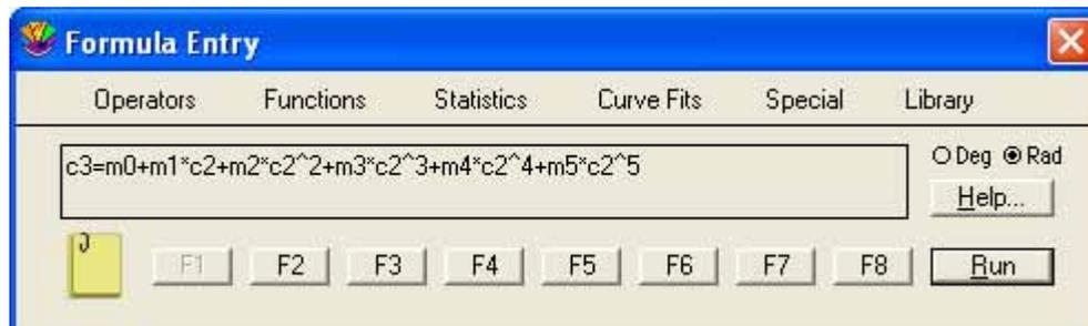
Figure 9-24 Using the curve fit equation to calculate values
