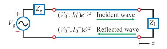
The presence of two waves on the line propagating in opposite directions produces a *standing wave*.
