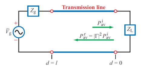
$$V_0^+ = \left(\frac{\widetilde{V}_g Z_{in}}{Z_g + Z_{in}}\right) \left(\frac{1}{e^{j\beta l} + \Gamma e^{-j\beta l}}\right).$$
