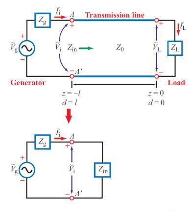
At input, d = l:  $Z_{in} = Z(l) = Z_0 \left[ \frac{1 + \Gamma_l}{1 - \Gamma_l} \right]$ .
