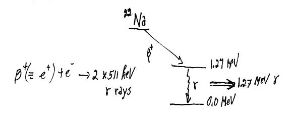
Fig. 5. <sup>22</sup>Na decay scheme
