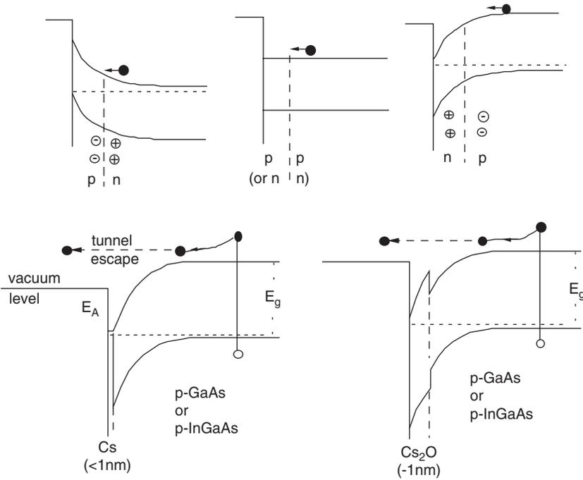
**Figure 4.** Band bending at the photocathode surface: a  $p$ -type surface layer atop on an  $n$ -type substrate curves the bands upward, hindering emission. An  $n$ -type layer on a  $p$ -type substrate curves the bandwidths downward, easing the emission of the electron from the conduction band to the vacuum by tunneling. The effect, called NEA (negative electron affinity), is taken to advantage in cesiated photocathodes.
