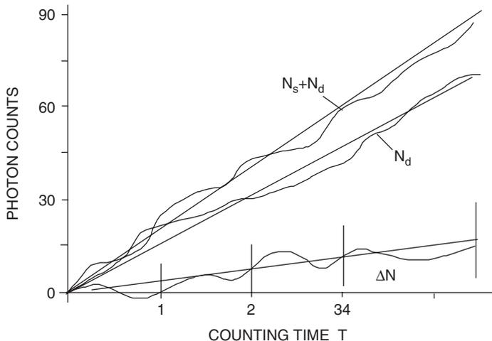
Figure 14. Basic functional scheme of photocounting (top), and an example of measurement, showing evolution of signal plus dark, dark only, and result after dark subtraction (bottom). Vertical bars on ΔN indicate the ±0.5σ<sub>Δn</sub> confidence level. (from Ref. 1, reproduced with permission of Prentice-Hall).
