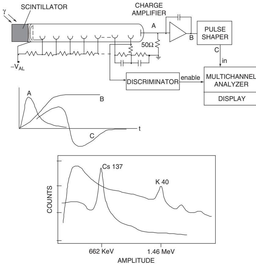
**Figure 15.** Scheme of energy spectrometry measurements (top) and signal waveforms (middle). The energy spectrum measured with the scintillation detector (bottom) reveals radionuclides species (energy signature) and their concentrations (counts intensity) (from Ref. 1, reproduced with permission of Prentice-Hall).
