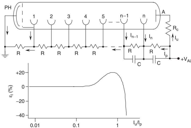
**Figure 13.** Schematic of the dynode voltage divider (top) and linearity error in dc current near saturation (bottom) (from Ref. 1, reproduced with permission of Prentice-Hall).
