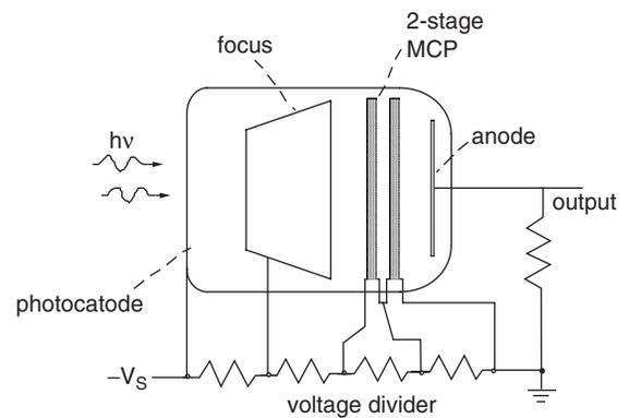
**Figure 9.** A two-stage MCP photomultiplier.
