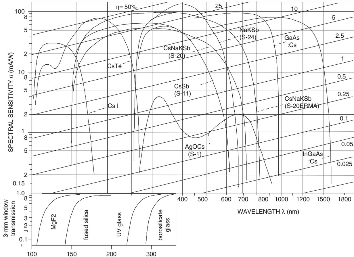
**Figure 5.** Spectral sensitivity  $\sigma(\lambda)$  vs. wavelength of reflection photocathodes. Lines of constant quantum efficiency  $\eta$  are also shown. The EIA standard designations are indicated in brackets. Inset shows the cutoff of common window materials (adapted from Ref. 1, with permission of Prentice-Hall).
