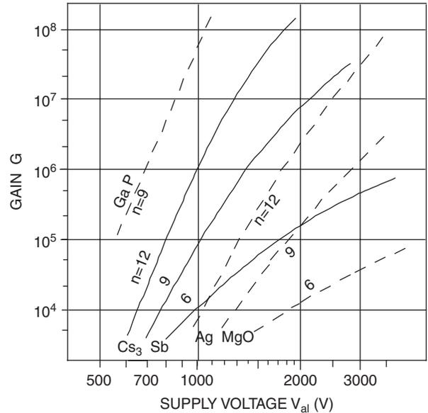
**Figure 11.** The gain of the dynode chain as a function of supply voltage for some commonly used dynode materials and number of stages (from Ref. 1, reproduced by courtesy of Prentice-Hall).
