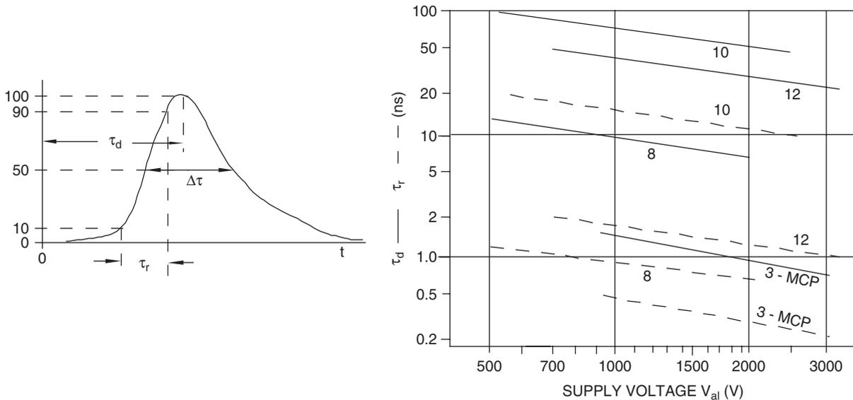
**Figure 12.** (left) Definition of the SER characteristic time parameters and, (right) the SER rise time  $\tau_r$  (dashed lines) and delay time  $\tau_d$  (solid lines) of typical PMTs, as a function of the total supply voltage, and with the number of dynodes as a parameter. (From Ref. 1, reproduced with permission by Prentice-Hall).
