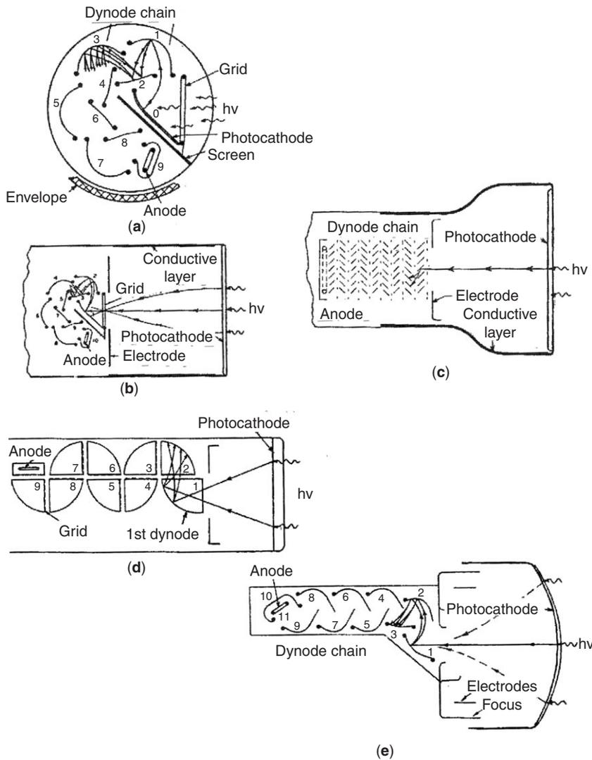
**Figure 7.** PMT structures: (a) squirrel-cage for reflection photocathodes and (b) for transmission photocathodes; (c) venetian-blind dynodes; (d) box and grid; (e) linear dynode-chain (adapted from Ref. 2, by courtesy of Burle Technologies).
