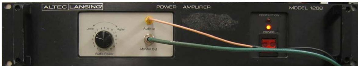
The power amplifier driving the AC magnet coils is an Altec Lansing stereo amplifier modified for single channel use with input and monitor connections on the front panel.
