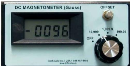
The AlphaLabs DC Magnetometer uses a Hall effect probe that is placed between the two magnet poles to measure the DC magnetic flux.
