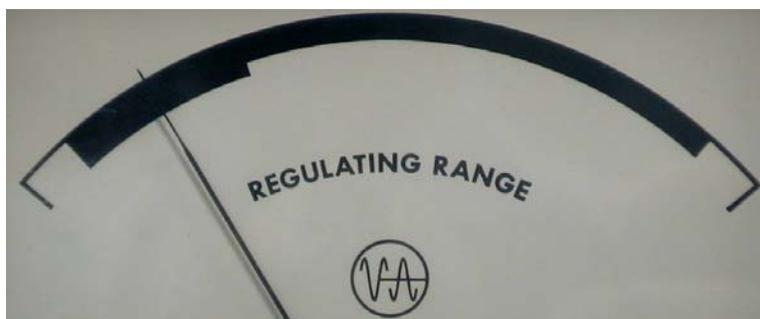
This indicates the correct operating voltage being dropped across the series pass regulator tubes. To the left of the darkest band you will lose magnet current regulation. To the right of the darkest band is another dark band in which regulation will still occur, but this is not an optimum regulating point. To the far right beyond the dark bands the pass tubes will be operating at too high a power level and might be damaged. *IN NO CASE SHOULD YOU LET THIS METER GO OFF SCALE ON THE RIGHT*
