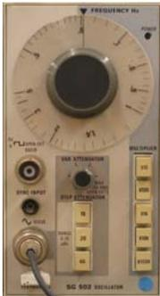
The Tektronix SG 502 Oscillator plugs into a Tektronix TM Power Supply Mainframe and feeds audio sine waves to the audio power amplifier.
