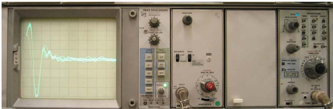
The horizontal sweep can be generated by triggering the time base internally (Display Mode-Time Base, Triggering Source-Internal) using the modulation signal from the Vertical Amplifier. This technique is helpful if an accurately linear scale is needed on the scope screen, such as measuring timing of the wiggles.
