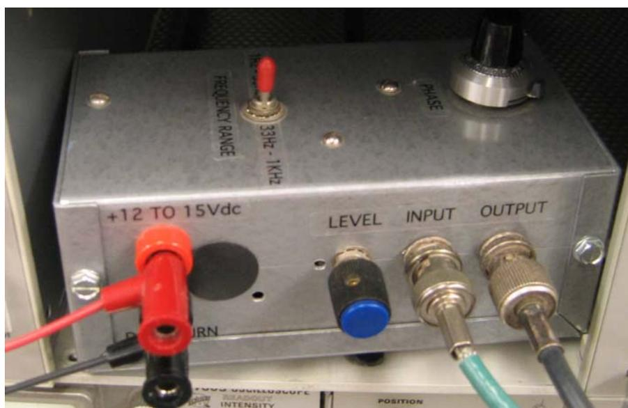
The **Phase Shifter** box has both a level control and a phase control. The level control is adjusted to obtain a full horizontal scan on the CRT and the phase control is adjusted to align the opposite scan waveforms.
