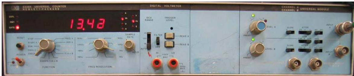
A Hewlett Packard 5328A Frequency Counter monitors the frequency of the RF oscillator to determine the actual frequency of an observed NMR signal.
