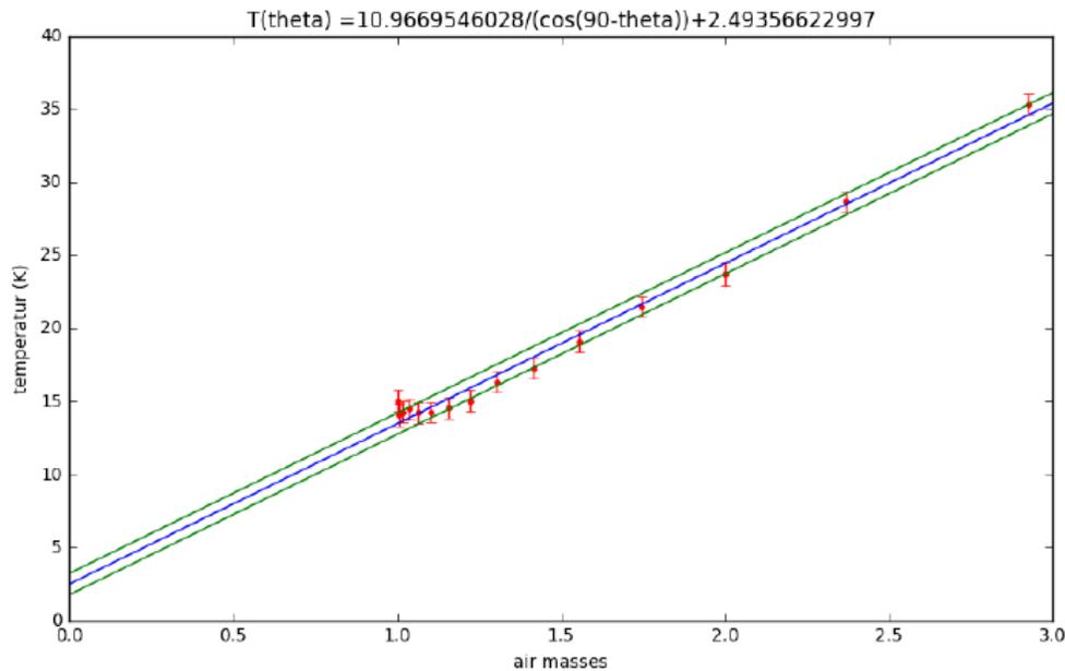
**Figure 12:** Estimating CMB noise temperature. This is an example of a student’s plot of data (eqn 7) obtained for a single run of measurements of temperature vs airmass. You may wish to choose a different zenith angle sampling scheme. Chi-sq fit extrapolated to zero airmass gives the estimated CMB temperature & error.
