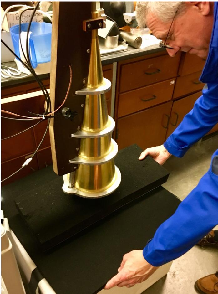
**Figure 8:** Cold and warm loads for calibration. The 19 GHz horn is shown pointing at the cold microwave absorber load immersed in liquid nitrogen inside the white styrofoam box, and the room temperature Eccosorb load is being placed in the beam. Calibrated diode thermal sensors in the edges of the loads report accurate load temperatures to the data acquisition system and are displayed on the Lakeshore meter.
