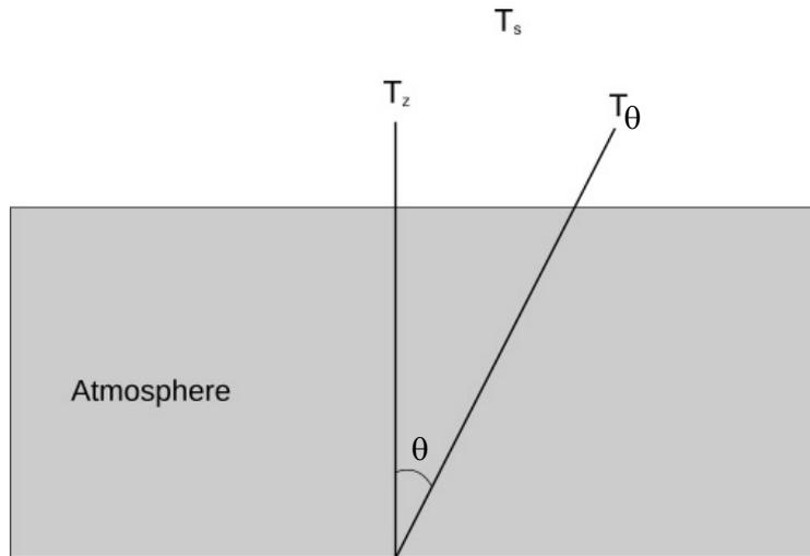
**Figure 10:** Calculating atmospheric noise. The intensity measured at an angle  $\theta$  ( $T_\theta$ ) will be higher than the intensity measured at the zenith ( $T_z$ ) due to more atmospheric emission microwave noise. Assuming the magnitude of atmospheric noise is a direct function of distance the signal travels through the atmosphere, we can calculate it using a measurement at the zenith and one at an arbitrary angle  $\theta$  to find the sky temperature  $T_s$ .
