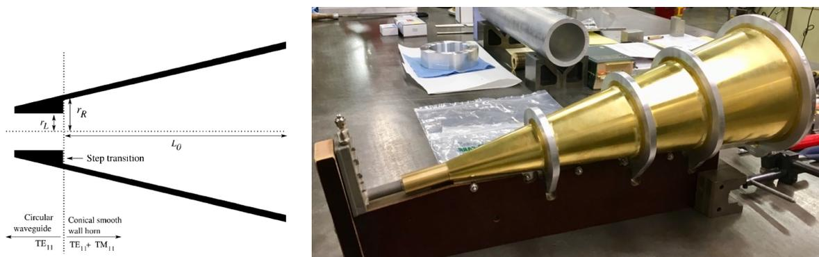
**Figure 3:** Potter horn antenna. Radiation from the sky is received by a specially designed horn, which has a narrow beam so that you can selectively observe various sections of the sky. This enables distinguishing the CMB from the atmosphere and the surroundings. The horn achieves its narrow beam by exciting other modes in the throat section (*left*) which cancel sensitivity at large angles (side lobes), creating a narrow beam shown in figure 4.
