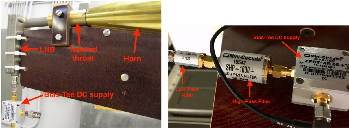
**Figure 6:** Radiometer electronics. On the *left* is shown the LNB mounted on the horn support. The Bias-Tee powers the LNB by routing a DC voltage through its output. Also shown is the special tapered throat and horn arrangement. On the *right* is shown the IF output of the LNB feeding (after the Bias-Tee) a 1000-1500 MHz band-pass filter composed of a 1000 MHz high-pass filter in series with a 1500 MHz low-pass filter.
