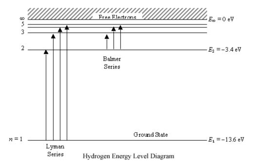
Figure 1. Energy-level diagram of the hydrogen atom according to the simple Bohr theory.
