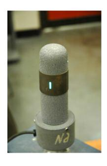
The Hydrogen-Deuterium light source is used with an external high voltage (5000 VAC) power supply. All electrical contact points are insulated, but care should be exercised in its use, and the power supply should always be turned off before handling the source lamp. This source will be used for taking the actual experimental data. **Be sure to turn on a fan aimed at the lamp.** Otherwise the tube will overheat and the line emission intensity will drop.
