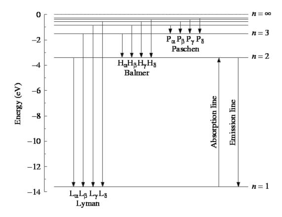
Figure 2. Transitions between the energy levels of a hydrogen atom. The lines  $L_{\alpha}, L_{\beta}$ , etc., belong to the Lyman series,  $B_{\alpha}, B_{\beta}$ , etc., to the Balmer series, and  $P_{\alpha}, P_{\beta}$ , etc., to the Paschen series, and so forth.
