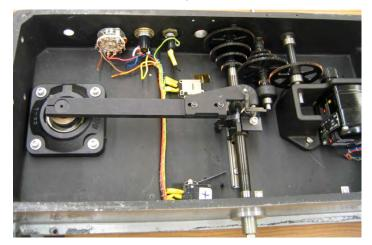
The easiest way to do a scan through a line or doublet is to run the monochromator to the short wavelength end of a narrow wavelength band spanning the line or doublet, beyond the first spectral line of interest and then scan back in the opposite (increasing wavelength) direction. You can experiment with the various power and manual scan speeds to find out what works best for you.
