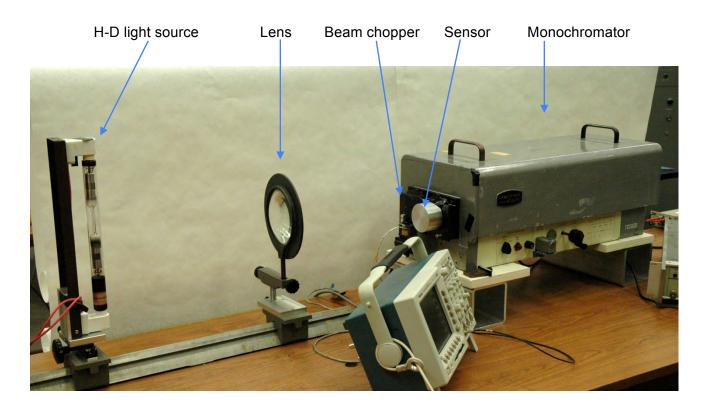
In the upper left is Hydrogen light source. Light is focused by the lens into the inlet slit on the left end of the monochromator and passes back through the exit slit into the aluminum box housing the photodiode light sensor. The sensor output is amplified and sent to the lock-in amplifier, off the image to the right.
