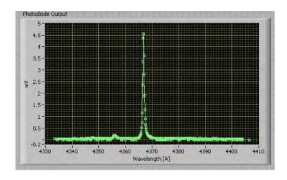
Using the 15µ slits, manually scan *towards increasing wavelength* along the monochrometer's range noting the wavelengths where the line peaks occur. Take this data and match it to the known line wavelengths to create the dispersion curve for the monochromator. Our test run for both scan directions provided the data below with dispersion values and chart – note the effect of back-lash in the gears. Your data may look different due to periodic maintenance of the monochromator.
