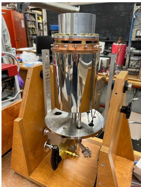
Fig. 1. Left: inverted cryostat with the outer chamber wall removed. Right: the inner sample chamber with the cap removed.
