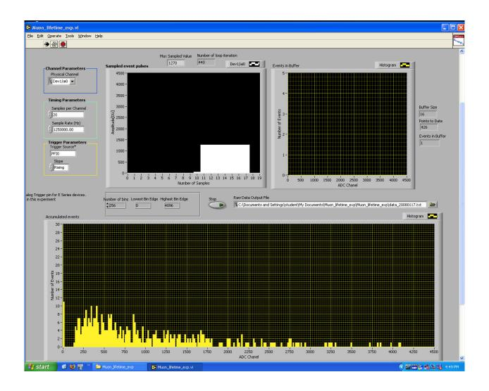
The display for the muon lifetime PHA GUI after only a couple hours of run time. The amplitude of the output of the Time-to-Amplitude-Converter (TAC) for each decay event is sampled (12 bits) by the Data Acquisition (DAQ) card and displayed at the bottom on the x-axis as 0-4096 (0-10  $\mu$ sec.) This screen shot shows the distribution of 530 decay events. Clearly a longer run time is needed for good statistics.
